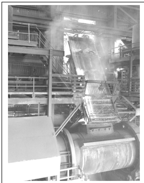
Figure 3 - PS converter technology and associated fugitive emissions
