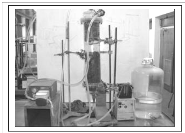
Figure 8 - Photo showing pack bed reactor at the CSIR
