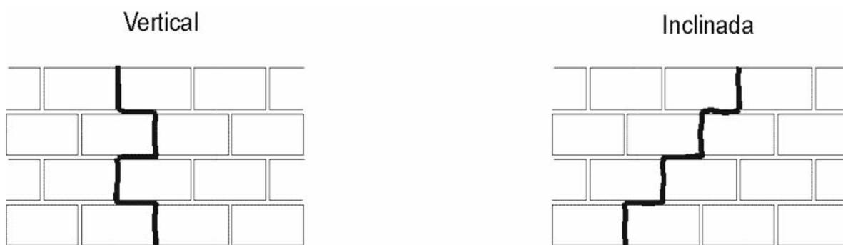
Figura 6 – Fissuras vertical/ inclinada
