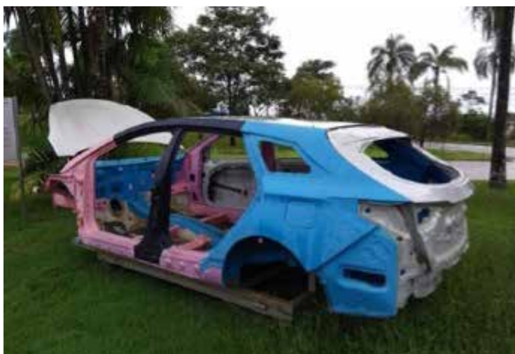
Figure 12. Vehicle body showing the different types of steels with niobium.
