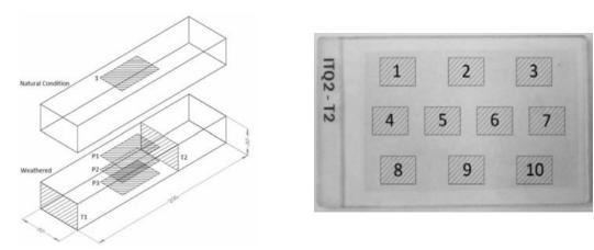
Fig. 1 a) On Left: Cutted areas from the specimens to obtain thin sections. b) On right: Position of pictures taken from thin section for image analysis.
