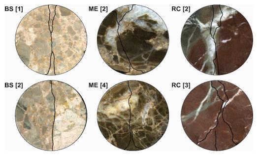
Fig. 1 Studied ornamental stones: Beige Serpiente (BS), Marrón Emperador (ME) and Rojo Cehegín (RC). Black lines drawn inside the samples correspond to the trace of the fractures developed after Brazilian test.
