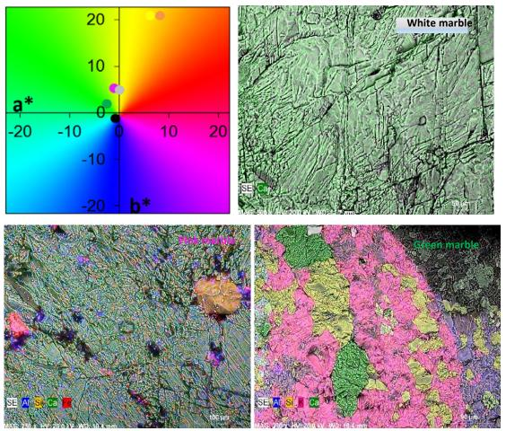
Fig. 2 Colour of the white, pink and green marbles and the compositional mapping by SEM. EDS in each sample.
