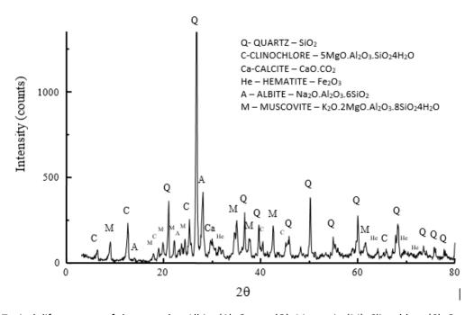
Fig. 1 Typical difractogram of slate powder: Albite (A), Quartz (Q), Moscovite(M), Clinochlore (C), Ortoclase (O) e Hematite (He).
