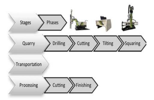
Fig. 1 Steps and stages on stone extraction with Fravizel prototypes. Source: Frazão and Frazão, 2013
