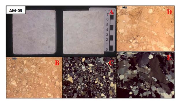
Fig. 3. **A)** AM-03 specimen for the Amsler abrasion test and macroscopic description; **B)** Natural Light\_5x\_ e **C)** Plane Polarized Light\_5x\_Showing the great predominance of quartz; **D)** Natural Light\_5x\_ e **E)** Plane Polarized Light\_5x\_Characteristic undulatory extinction of quartz that is a feature of this lithology. *Qtz* → Quartz; *Fds* → Feldspar (PI e Kfs).
