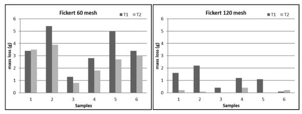
Fig. 3 Results of mass loss of the ecological fickerts after the polishing test.
