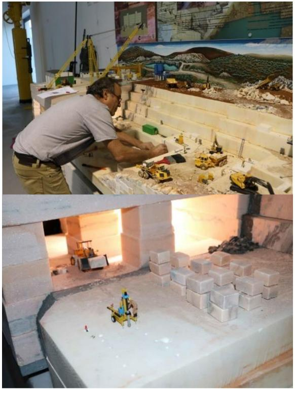
Fig.2 Assembly phase of the model and detail of the underground exploitation and drilling in open pit.
