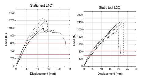
Fig. 1 Load-displacement curves for the static tests L1C1 and L2C1
