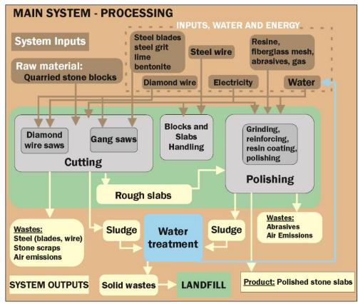
Fig. 1 Boundaries of the slabs production system (Main Product System).
