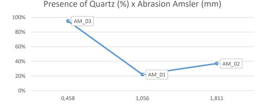
Fig. 4. Results of Amsler abrasion tests for sampled rocks.
