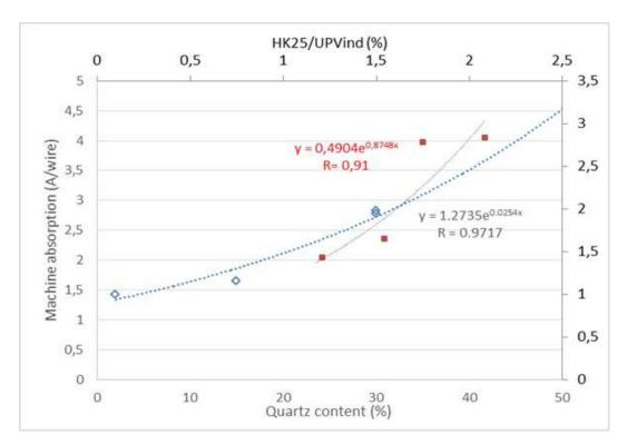
Fig. 2 Machine absorption vs H25/UPVind and vs quartz content for RBE, SIE, DIOs and GRP
