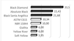
Fig. 6 Uniaxial compressive strenght (MPa).
