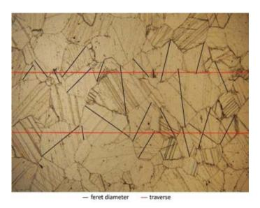
Fig. 2 Linear traverse method for determination of the grain size distribution
