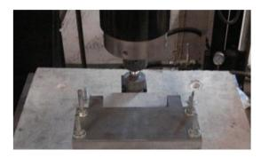
Fig. 1 Test to determine resistance at the anchor point for pin-type metallic inserts.
