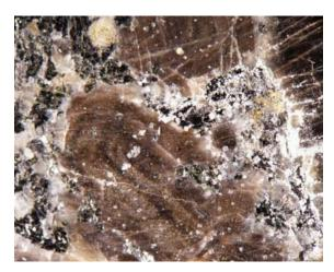
Fig. 1. Halite crystals on the polished surface of Imperial Brown Granite. Small crystals with average size of 1mm on feldspar surface and on surrounding grains.
