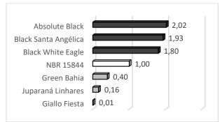
Fig. 7 Thermal Expansion ( $10^{-3}$  mm/ $^{\circ}$ C).
