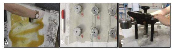
Fig.2 Example of application of the resin on the stone sample: (A) Sample ready for the test and (B) Reading of breaking load by the pulling device (C).
