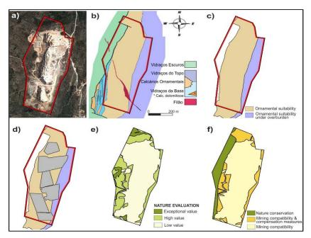
Fig. 3 Results from the geological and environmental studies carried out at the Cabeça Veada site: a) aerial view of the quarrying site; b) geological thematic mapping; c) delimitation of the suitable areas for limestone quarrying; d) existing licensed quarries; e) GIS integration of the natural values evaluation process; and f) land use spatial planning proposal for the Cabeça Veada site.
