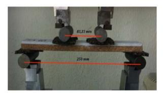
Fig. 2 Distance between supports for the bending test.
