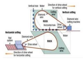
Fig. 2 Cutting Process in the extraction of stone bench. Source: Bagherpour, Khademian, Almasi and Aalaei (2014)
