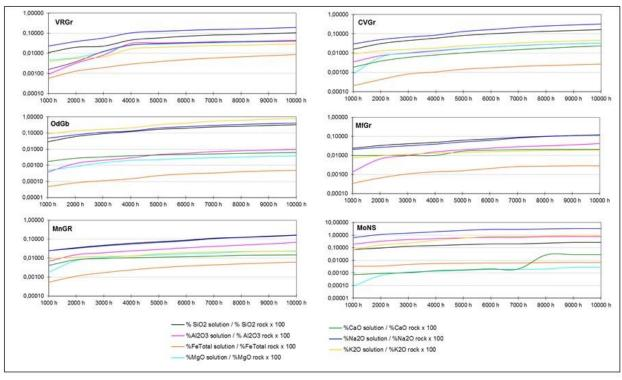
Fig. 1 Accumulated variation for Si, Al, Fe, Mg, Ca, Na and K (major elements oxides) in the cycles of the Soxhlet experiment waters.
