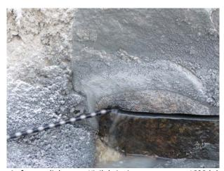
Fig. 2 A horizontal wire cut in frozen diabase at Kivilahti, air temperature -18°C (photo 12<sup>th</sup> December 2016).
