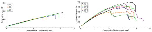
Fig. 1 Load displacement curve a) for BAS specimens b) for WGA specimens
