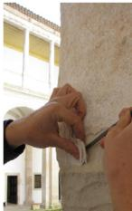
Fig. 1 Monastery of Santa Maria of Alcobaça (Portugal), left and loss of cohesion in the limestone in Cloister of "Hospedaria", right.
