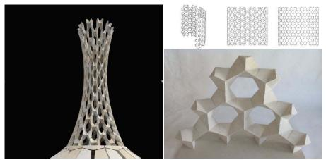
Fig. 2: "Alveare" project. Left, perspective of the final structure idealized by the group. The smaller modular piece, better seen in the picture at right, can be parametrically deformed and used to build infinite types of shapes. (From: FALLACARA, G. New Fundamentals of Natural Architecture, 2014)
