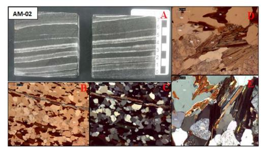
Fig. 2. **A)** AM-02 specimen for Amsler abrasion test and macroscopic description; **B)** Natural Light\_5x\_e **C)**Plane Polarized Light\_5x\_showing lepdoblastic texture; **D)** Natural Light\_10x\_ and **E)** Plane Polarized
