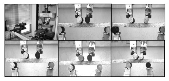
Fig. 1 VIC test a) Test apparatus; b) L=2S/11, S=250mm; c) L=S/3, S=250mm; d) L=S/3, S=200mm; e) L=S/3, S=150mm; f) L=S/3, S=100mm
