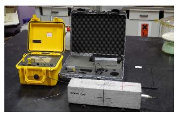
Fig. 1 Resonance Frequency meter 58-E0035/C.
