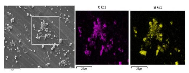
Fig. 4 EDS mapping of slate waste.
