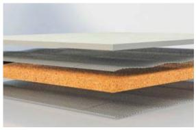
Fig. 1 Stone and cork sandwich-structured composites schematic representation.
