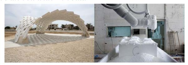
Fig. 1 LEFT: Stone Matters, prototype 01. The use of stereotomy – the process of cutting stones – to make contemporary architecture. Fig. 1 RIGHT: Stone Matters, prototype 01. Milling Styrofoam with a robotic arm, aiming to do a negative form of the vault's centre. (From: <a href="http://aauanastas.com/project/stone-matters/">http://aauanastas.com/project/stone-matters/</a>)
