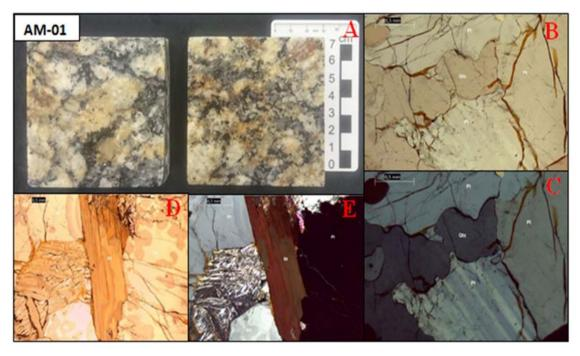
Fig. 1. A) AM-01 rock sample used for the Amsler abrasion test and macroscopic description; B) Natural Light\_5x\_ and C) Plane Polarized Light\_5x\_showing the predominance of quartz in the thin section; D) Natural Light\_5x\_ and E) Plane Polarized Light\_5x\_ showing the presence of Biotite and Chlorite.  $Pl \rightarrow$  Plagioclase;  $Qtz \rightarrow$  Quartz;  $Bt \rightarrow$  Biotite e  $Chl \rightarrow$  Chlorite.
