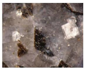
Fig. 2. Halite crystals deposited on the polished surface of Labrador Brown Granite after 10 years rest. The largest crystal is 5mm. long in diameter.
