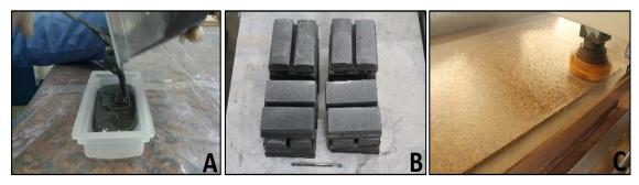
Fig. 2 Fickert molding process (A), fickert samples (B) and polishing test (C).
