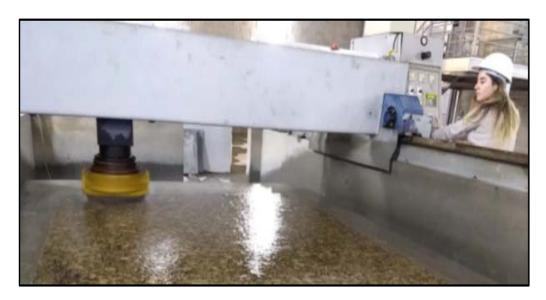
Fig. 2. Polishing running test of the dimension stone slab in semi-automatic polishing machine.
