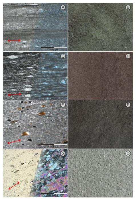
Fig. 1 Petrographic (left column) and hand specimen images (right column) of the lithotypes of roofing slates. In the left column, the right part of the picture uses crossed polarizers. The red line marks the direction of the cleavage.
