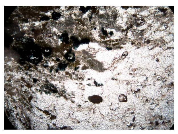
Fig. 3. Photomicrography of the Imperial Blue quartzite showing the contact between a hydrothermal venule with the quartzite matrix. Note the presence of rutile-associated tourmaline, monazite and muscovite. Tur = tourmaline; Rut = rutile; Qz = quartz; Mon = monazite; Leuc = leucoxênio.
