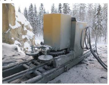
Fig. 4 Formation of ice on pulley and drive wheels. Photo was taken on 12<sup>th</sup> December, daytime temperature was -18°C. Wire saw unit is Huada 55 kW, powered by a diesel aggregate lwego 175 kW.
