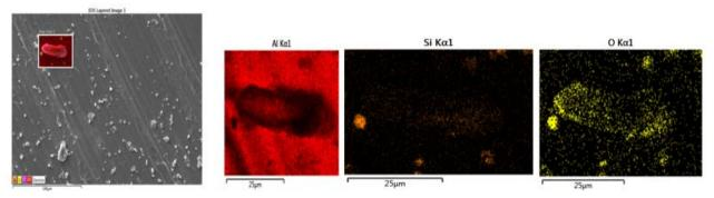
Fig. 5. EDS mapping of slate waste
