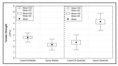
Fig.3 Results of tensile strength of marble resin with castor oil resin and epoxy resin (A)and Results of tensile strength marble resin with castor oil resin and epoxy (B).
