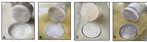
Fig. 4 After the test. Marble with epoxy resin (A) and castor oil resin (B) and Quartzite with epoxy resin (C) and castor oil resin (D).
